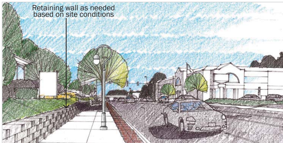
Streetscape Example: Adjacent Retaining Walls
